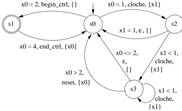
Figure 3. Automaton  $T$ : a simplified airplane control
